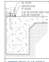
MONOLITHIC SLAB DETAIL
